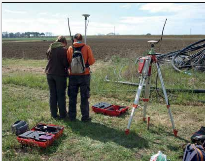
Fig. 2 - Topographic survey being conducted using a GPS with base station and rover (photo: K. Strutt).
