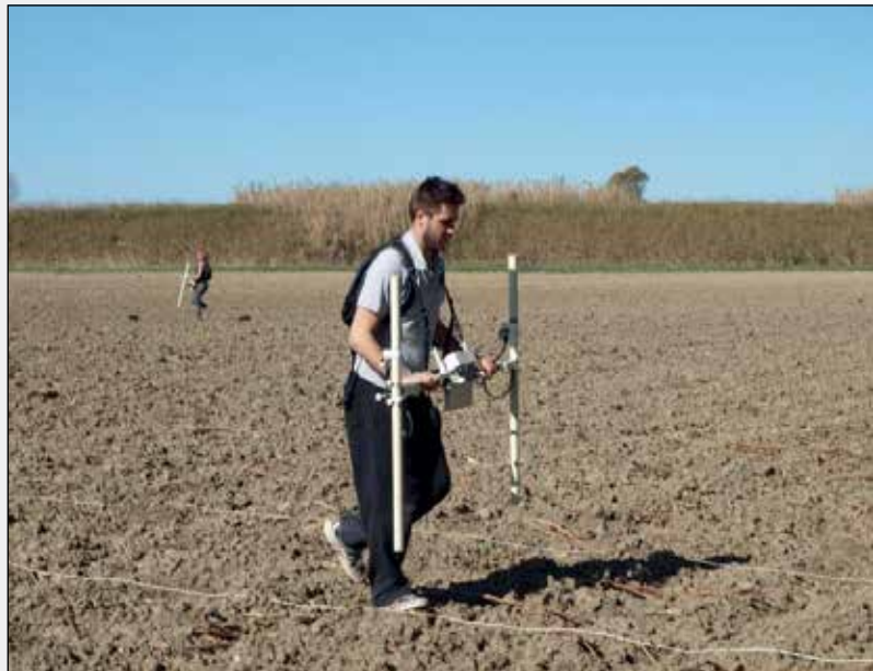
Fig. 1 - Fluxgate gradiometer magnetometry being carried out on the Isola Sacra (photo: K. Strutt).
